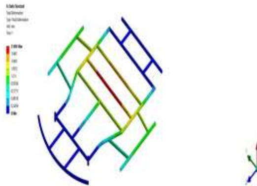
Fig.6 Torsional load displacement in ANSYS
